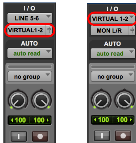
Pro Tools screen shots showing signals being digitally routed from the DAW into Console for monitoring and/or Realtime UAD Processing (left) and from Console into the DAW for recording and/or further processing (right)
