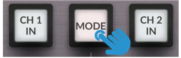
Press and hold the MODE key whilst The Bus+ is powering on
