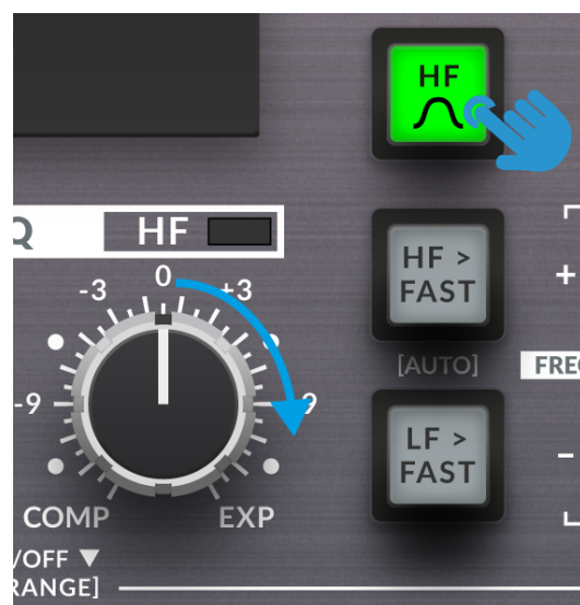
Press and hold the HF BELL switch until it turns green and then rotate the HF control clockwise to start expanding.
