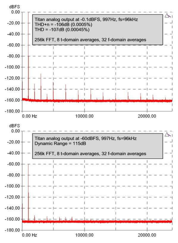
Except where otherwise stated, audio performance data are typical, RMS, unweighted, 20Hz..20kHz figures, measured at 997Hz, using fs=96kHz and '+4dBu' sensitivity settings.
