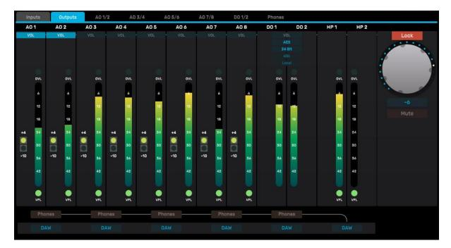
Line output level is switched between +4dBu and -10dBV nominal by the '+4/-10' radio buttons.
