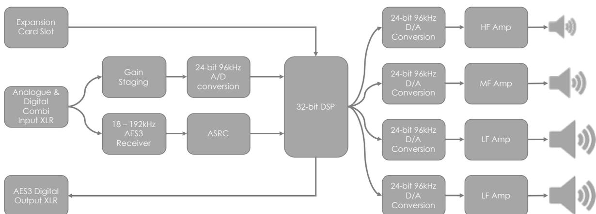
\* The diagram shows 4 channels of amplification, as used in the PMC6-2 and PMC8-2 models.
