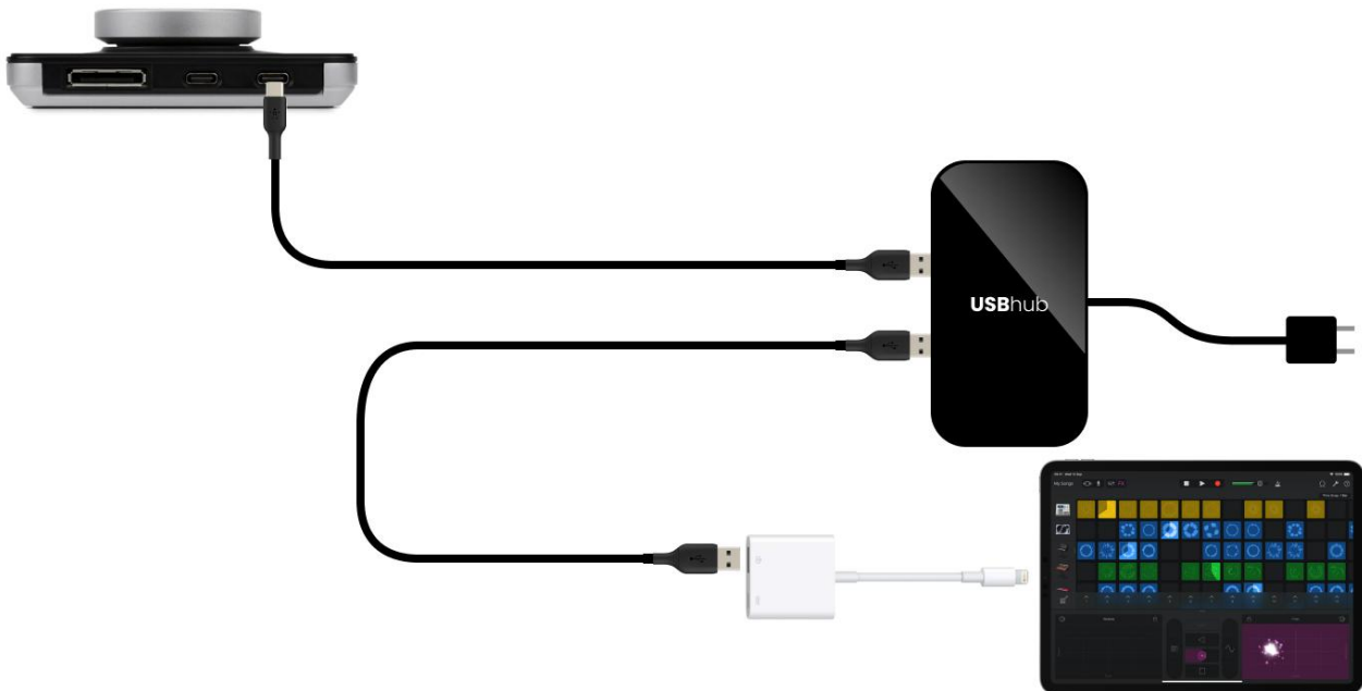
Connecting Duet 3 to an iPad with Lightning connector via powered USB hub/Camera Connector Kit
